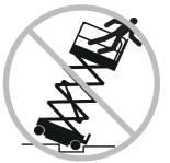
Use extreme care and slow speeds while driving the machine in a stowed position across uneven terrain, debris, unstable or slippery surfaces and near holes and drop-offs.
